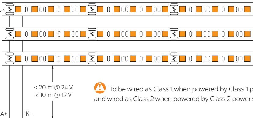
⚠ To be wired as Class 1 when powered by Class 1 power supply
