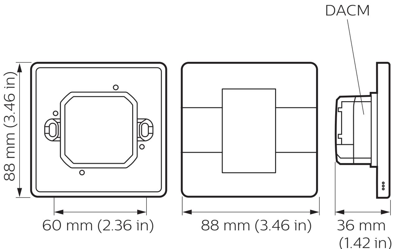
\* The mounting plate must be grounded to avoid field effect false triggering by nearby ungrounded metal objects.
