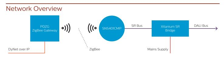
Warning - This device connects to an SR bus only. Do not connect directly to a DALI bus.
