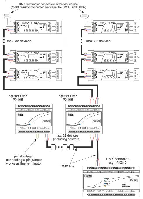
c) shorting of 120R pins – if the splitter is the last device and no receiver is connected to the *DMX THRU* output, the bridge on these pins acts as a terminator
