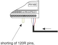
shorting of 120R pins, (works like connecting a terminator, if the splitter is the last device)
