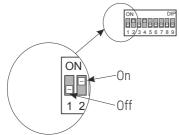
White color shows position of the switch. In upper position DIP switch is ON and in lower position it is OFF.
