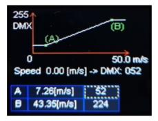
Parameter A and B is the wind speed, adjustable from 0 to 50[m/s]. By default, parameter A is set to 0 [m/s] and the value DMX 0, while parameter B to 50 [m/s] and DMX to the value 255.
