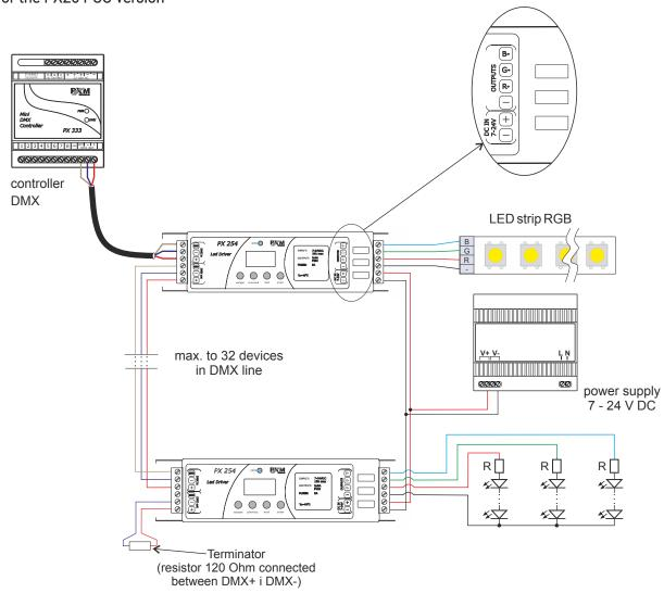
Note! The driver PX254-CC is common cathode type device. It is possible to connect lamps with 4-wires cable with a common "-" only.
