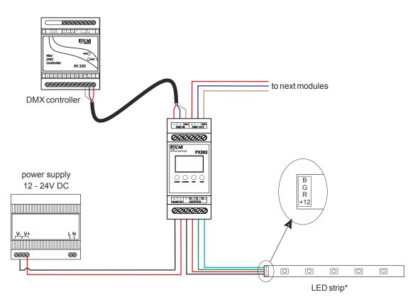
\* typical LED strips are supplied with 12V DC – then the PX282 has to be connected also the 12V DC power supply with adequate power, in the case of using LED strips supplied with 24V DC, the PX282 has to be connected to 24V DC power supply that power is matched to the length of the strip.
