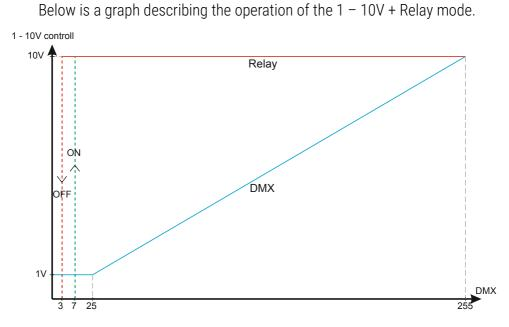
A DMX value of 0 corresponds to a voltage of 1V, with a DMX value of 25 starting to increase linearly to a value of 255. Relay switch is turned on by hysteresis, with DMX value 7 (and more), while DMX 3 value (or less) turns Relay off.
