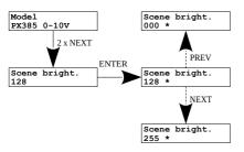
100%. Value 128 means the stage brightness is 50%. After changing the value of the stage brightness, the operation has to be confirmed by pressing *enter* or *escape*.
