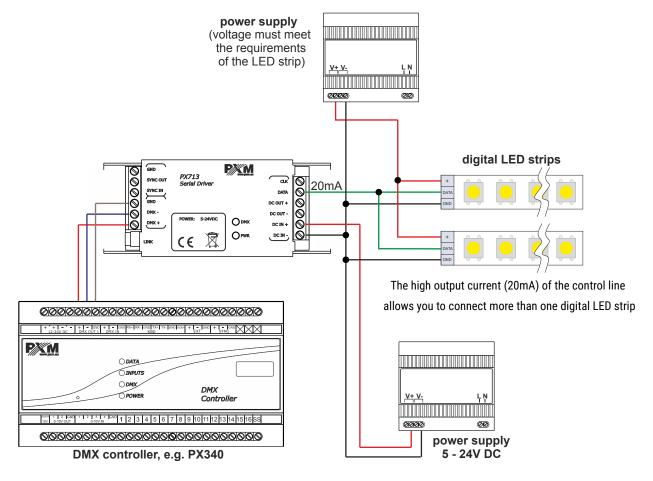
Connecting power from one shared source to the digital LED strip and to the driver
