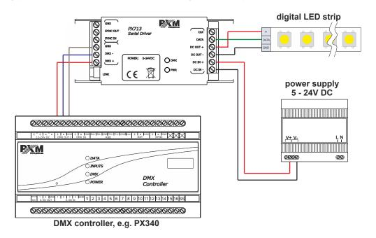
**NOTE!** The voltage of the power supply must be in accordance with the specifications of the digital LED strip. If strip must be powered by 5V DC, common power supply for the strip and the driver must be 5V DC!
