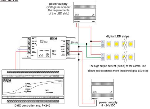
Connecting power from one shared source to digital LED strip and to driver digital LED strip
