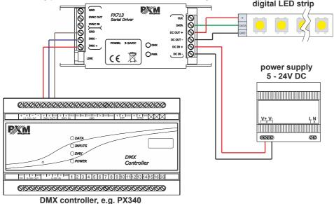
**NOTE!** The voltage of the power supply must be in accordance with the specifications of the digital LED strip. If strip must be powered by 5V DC, common power supply for the strip and the driver must be 5V DC!
