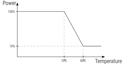
**NOTE!** After exceeding the upper temperature limit, the driver is not completely turned off, but the power is limited to 10%.
