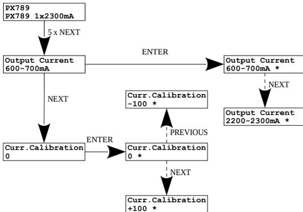
The chart below shows the *schematic* operation of the calibration option on the example for the ranges 700 – 800mA and 800 – 900mA.
