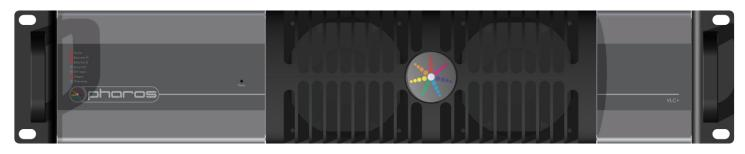
The Pharos VLC+ (Video Lighting Controller Plus) is designed to control the world's largest lighting façade projects. It renders multiple layers of effects and video from internal storage or live input, and features processing including rotation and masking. Up to 3,000 universes of eDMX and DVI-D can be output from a single unit with integrated show control.
